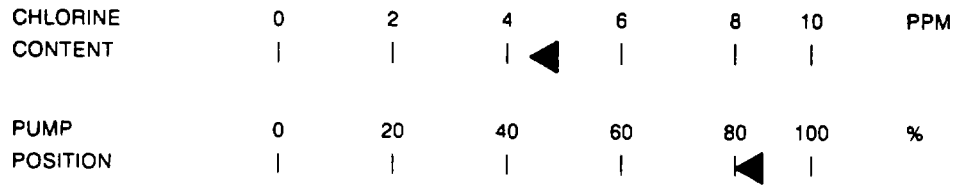
Figure 3-11. Chlorine Status Display Page
